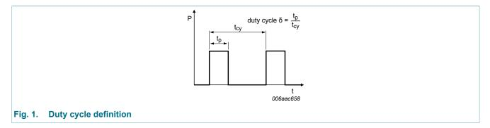
The current ratings for the typical waveforms are calculated according to the equations:  $I_{F(AV)} = I_M \times \delta$  with  $I_M$  defined as peak current,  $I_{RMS} = I_{F(AV)}$  at DC, and  $I_{RMS} = I_M \times \sqrt{\delta}$  with  $I_{RMS}$  defined as RMS current.
